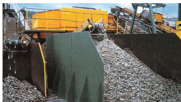
Non-ferrous metal separator used in combination with suspended magnetic separator installed in separating plant
